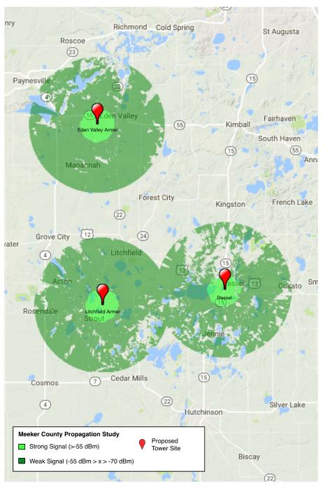
The wireless propagation studies in this section (as illustrated on the map on the previous page) look at the kind of wireless coverage and access that could be possible using proposed tower locations. The proposed tower locations listed below may not be the final locations for a wireless network. Further analysis including physical site surveys will be required to identify the final locations.
