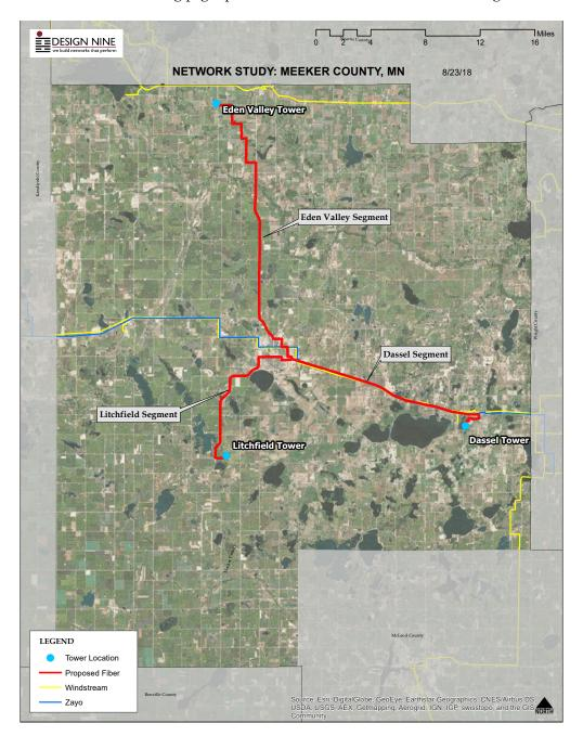
The diagram below shows the three towers and the fiber segments between each tower.
