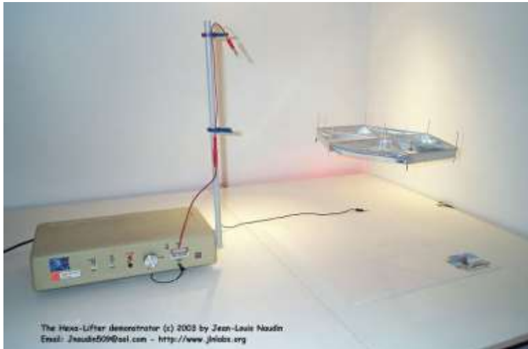
One of JL Naudin's "Hexalifter" experiments from 2003 66 . The lifter is tethered by 2 thin copper wires which provide the electrical power.
