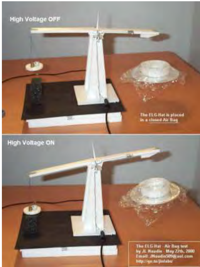
Experiment is repeated with “hat” inside a plastic bag, to reduce any “ion wind” effect.
