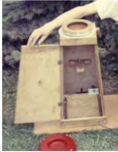
This photo shows the connection to the motor driving the rotor. The red disk-shaped object on the ground might have been used to cover the rotor, perhaps for safety and/or to hold an object to be levitated.
