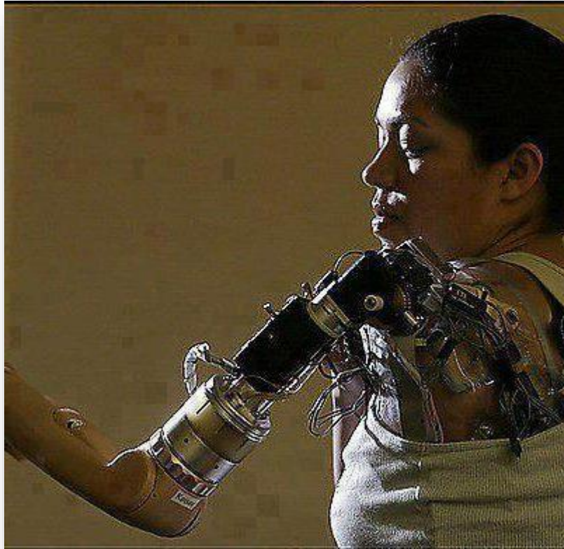
Figure 7. Claudia Mitchell, the first woman to have a "bionic arm", which follows the signals from the brain, just like a normal arm
