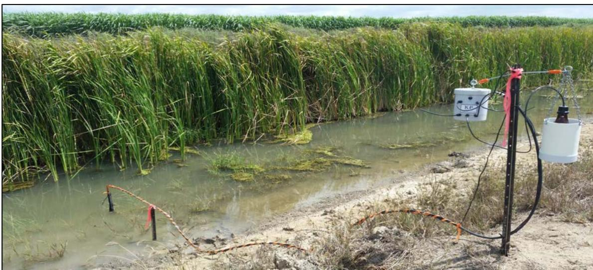
**Plate 3:** Water quality monitoring equipment installed at the wetland treatment system as part of project BSFF01. Source: BBIFMAC (2019).
