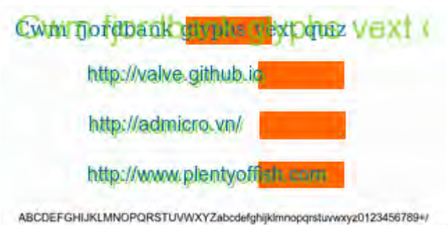
Figure 4: Different images printed to canvas by fingerprinting scripts. Note that the phrase “Cwm fjordbank glyphs vext quiz” in the top image is a perfect pangram , that is, it contains all the letters of the English alphabet only once to maximize diversity of the outcomes with the shortest possible string.
