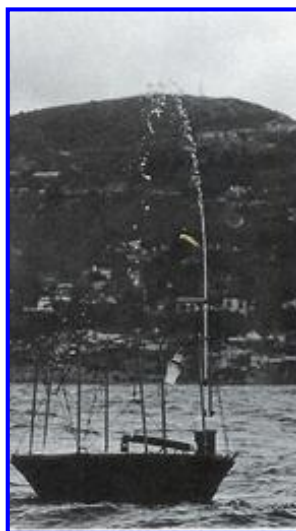
Middle: Wave pump testing off La Jolla, CA produces a stream 4m in light seas (photo S. Suess). Right: US Marine helicopter assisting wave pump deployment off Kaneohe Bay, Hawaii (photo US Navy). From Behrman1992, picture section , pictures © 1992 American Geophysical Union, Reproduced by permission of American Geophysical Union
