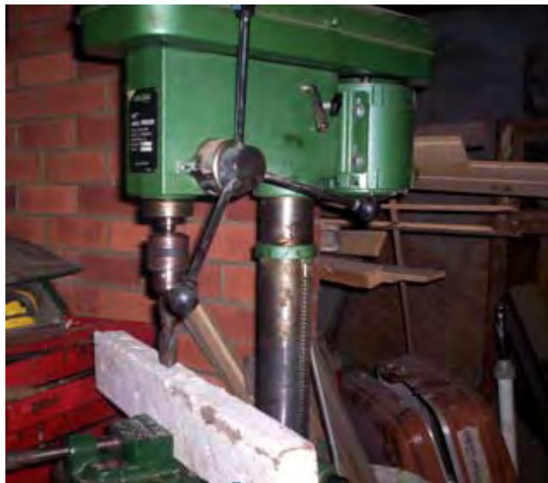
\frac{3}{4} Hp single phase Drill
