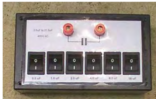
Values starting at 0.5uF [left] to 16uF [Right]
