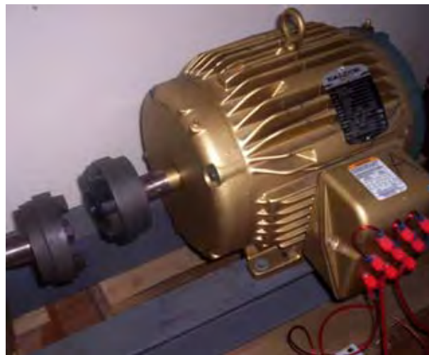
Panacea's Baldor motor EM3770T used for the RV Prime mover
