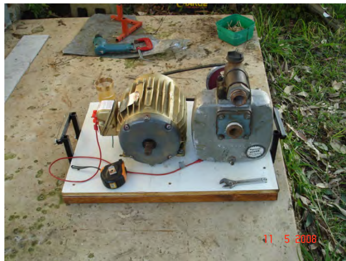
Above is Panacea's RV converted water pump with the external fan removed.
