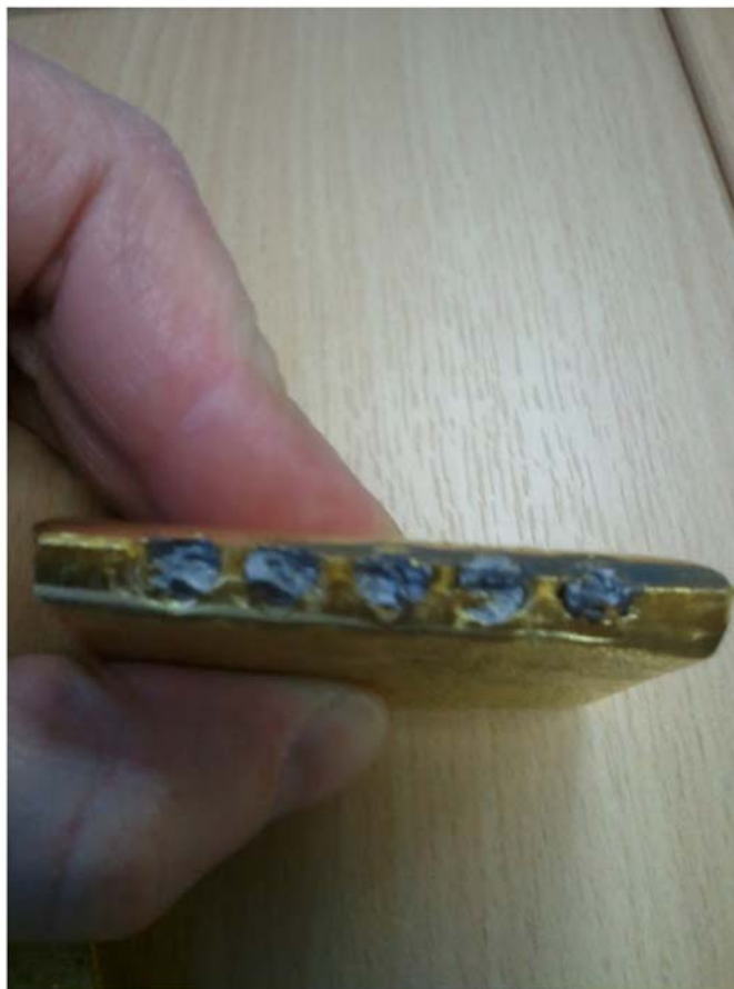
1000g Gold bar cut showing inserted tungsten rods
