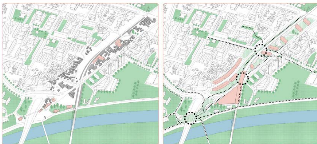
Figure 5: Urban structure of the analysed area before transformation (left) and the proposal for the new structure (right) with markings (black circles) of three proposed new pedestrian connections / public spaces establishing links between settlements: Savska – Prislavlje link in the north, Intermodal hub link in the middle and River Sava link in the south. source: Sladović, 2021.
