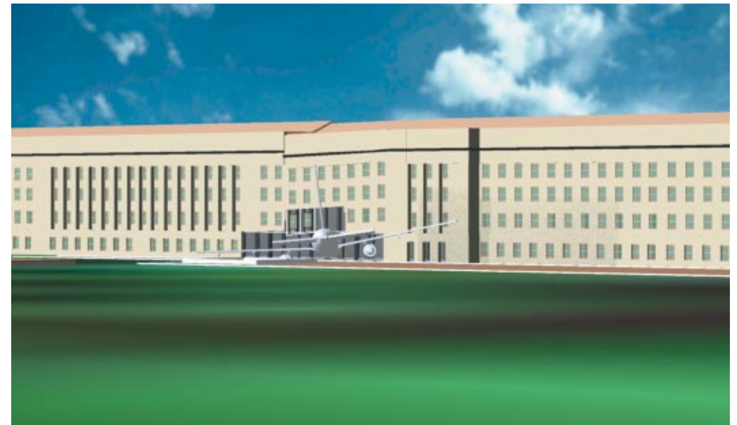
Figure 6.1 Aircraft aligned with damage on west facade
