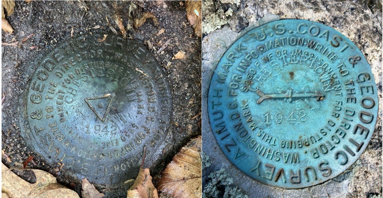
Triangulation marker (left) and azimuth marker (right) from the 1942 U.S. Coast and Geodetic Survey on Panther Mountain, with "CHESTERTOWN" stamped on it. (Credit: John Sasso)
