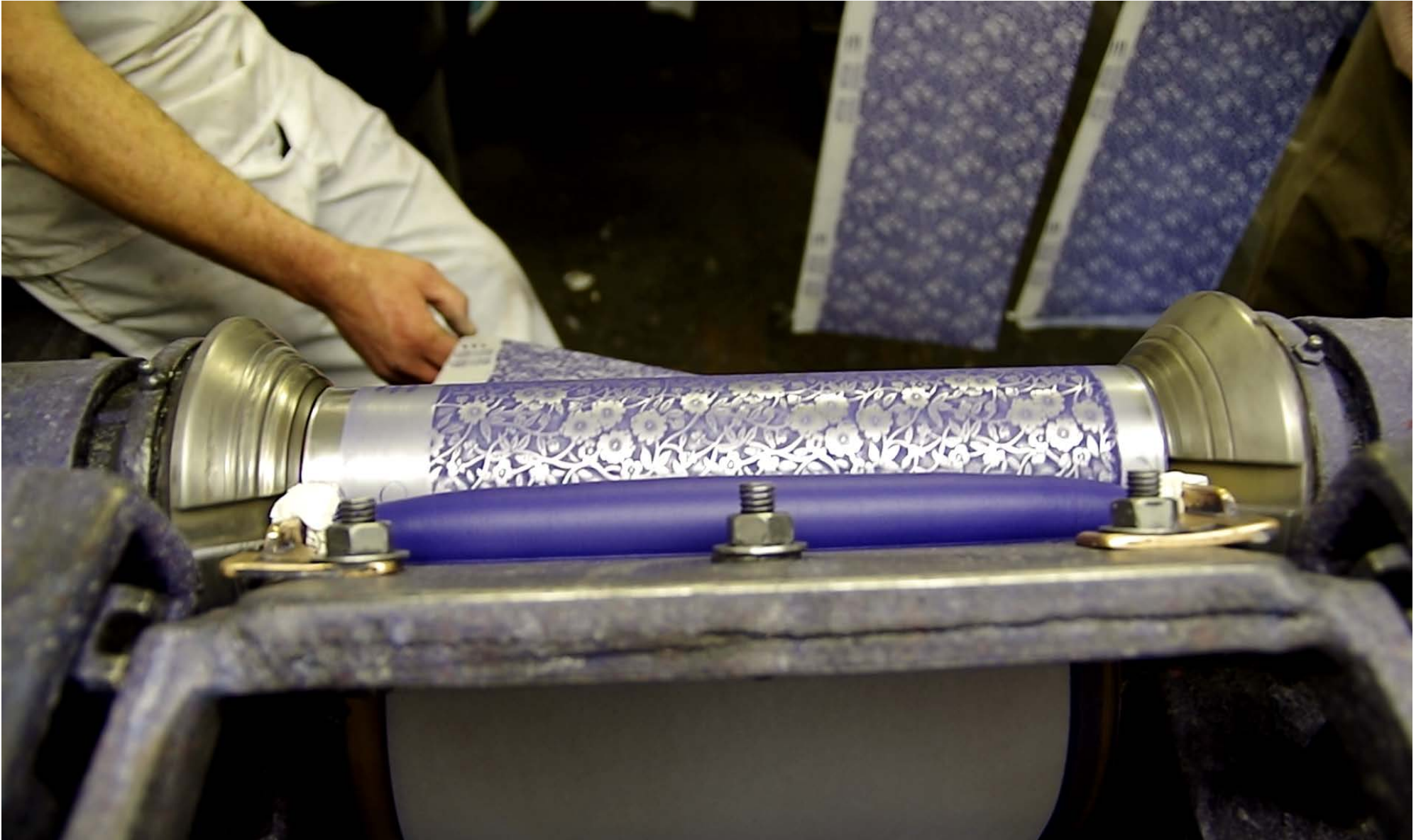
Printing from a copper roller at Burleigh
