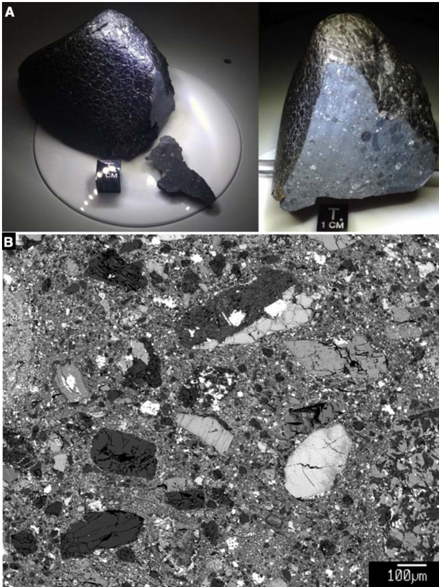
Fig. 1. (A) NWA 7034 hand specimen. (B) Backscatter electron image of porphyritic texture in NWA 7034. Large dark crystals are feldspar, large light colored crystals are pyroxene.. Portion of a gabbroic clast is shown above the scale bar.
