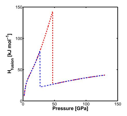
Fig. 4.— Dashed curve (red in the on-line version) is the enthalpy of fusion as a function of pressure for pure water (Goncharov et al. 2009). The branching in the melting curve, due to the super-ionic phase, is here at 47 GPa (Goncharov et al. 2005). Dashed-dotted curve (blue in the on-line version) is a hypothetical enthalpy of fusion, where, the branching in the melting curve occurs at 27 GPa.
