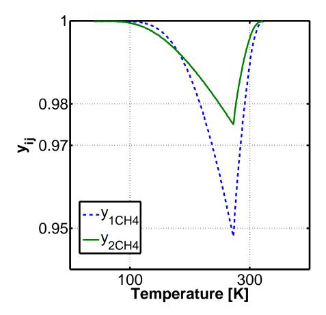
Fig. 6.— The probability of a methane molecule to occupy the large  $(y_{2CH_4})$  and the small  $(y_{1CH_4})$  cage of the structure I clathrate.
