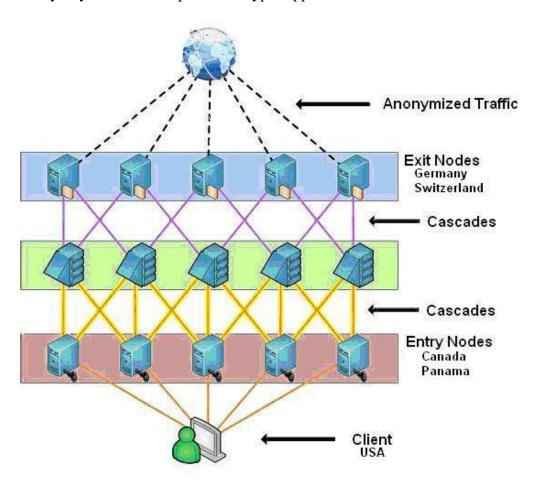
In this example, the client is in the US and a VPN tunnel runs from their computer to an entry node in either Canada or Panama, where the return address is also stripped-off. This means that a single surveillance operation is likely to lose the traffic here.
