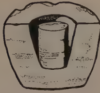
A bore-hole and core stem produced by tubular drilling during the Pyramid age (after Flinders Petrie).
