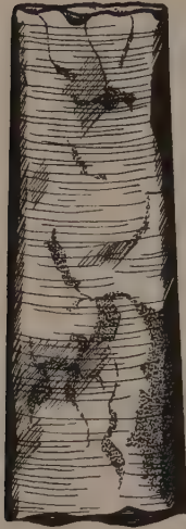
A granite core produced by tubular drilling in Old Kingdom times (after Flinders Petrie).
