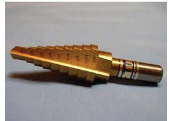
A step drill bit suited for drilling clean holes in plastics.
