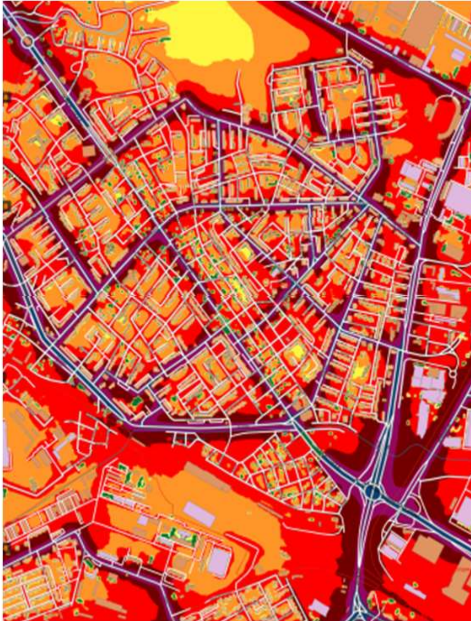
Figure 401.Noise levels from all sources for full day (Key: ten positions from green low levels(30 dB) to yellow, orange, red, violet- high levels (8dB and higher0), Source: http://www.isofmap.bg/ , http://www.gis-sofia.bg/bg/projects/gis-sofiya-eood-razrabotva-strategicheska-karta-na-shuma-v-stolitsata
