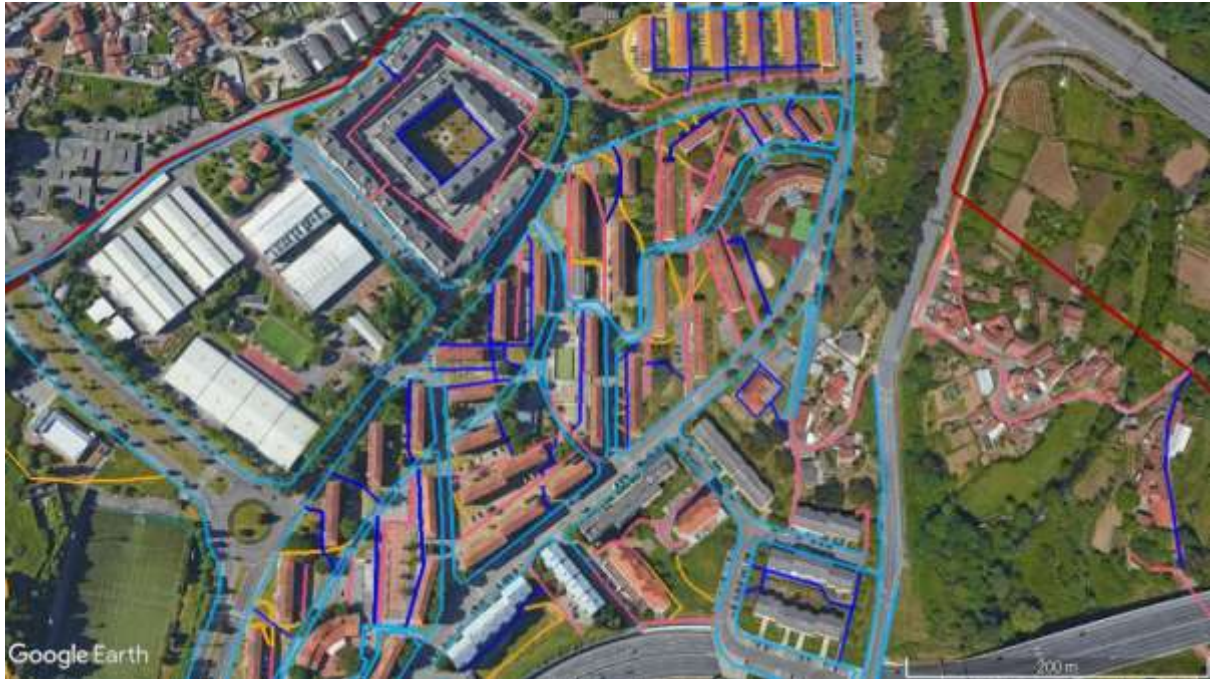
Figure 13. Case study of the application of the methodology in Porto (source: ICETA-CIBIO adapted from Google Earth). Legend: Sidewalks (Light blue lines); Shared roads (Pink lines); Pedestrian roads (blue lines); Informal Paths (Yellow lines); Bus stations (Bordeaux dots); Stage 2 study area polygon (red polygon); Crosswalks (green lines)
