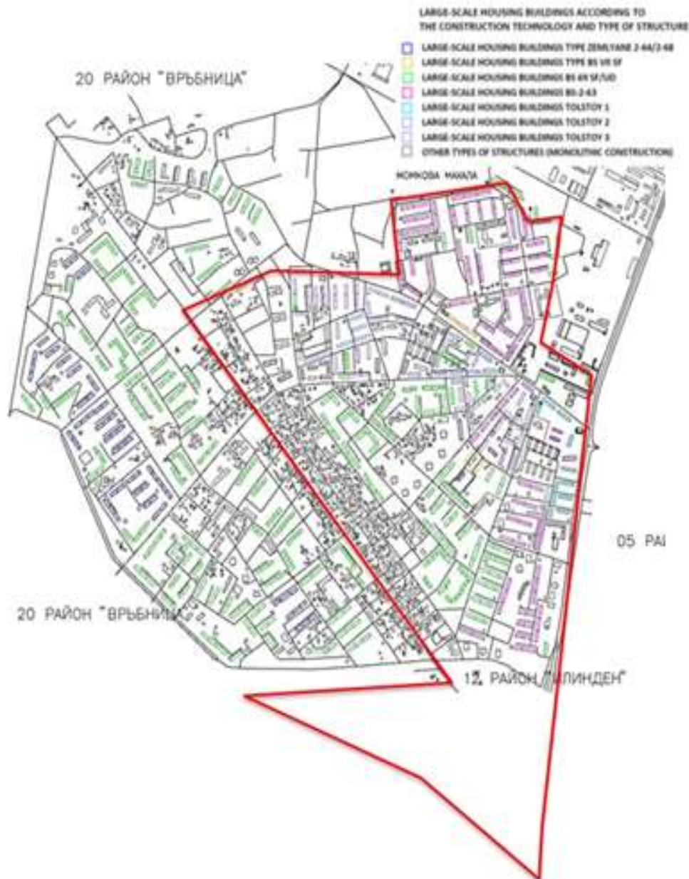
Figure 431. Types of pre-fab residential buildings by structure (industrialized) in Nadezhda district. Scheme modified for the purposes of URBiNAT. Source: Municipal programme for refurbishment and implementation of energy efficiency measures in the residential buildings in Sofia, Subregion 13 Nadezhda district.
