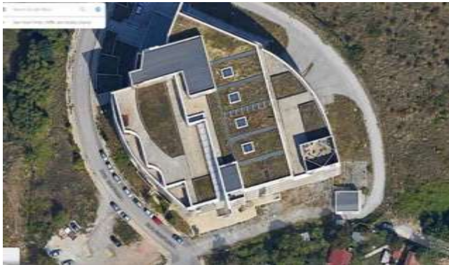
Green roof of an office building in the urban fringe, Source: Google Earth
