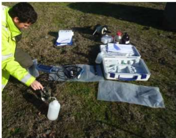
Figure 8 on-site measurement of water bulk physicochemical parameters
