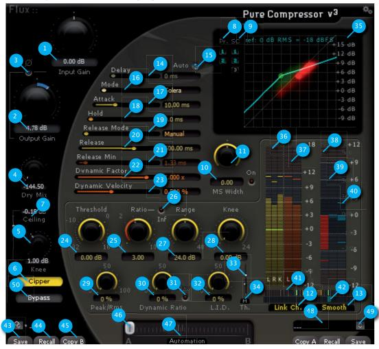
Pure Compressor is the compressor section of the Solera. A compressor is used to automatically reduce the gain above the Threshold. Pure Compressor produces a wide range of compressions from ultra clean subtle compressions to classic heavy pumping ones - It's all up to your artistic choices, not to the technology limitations.
