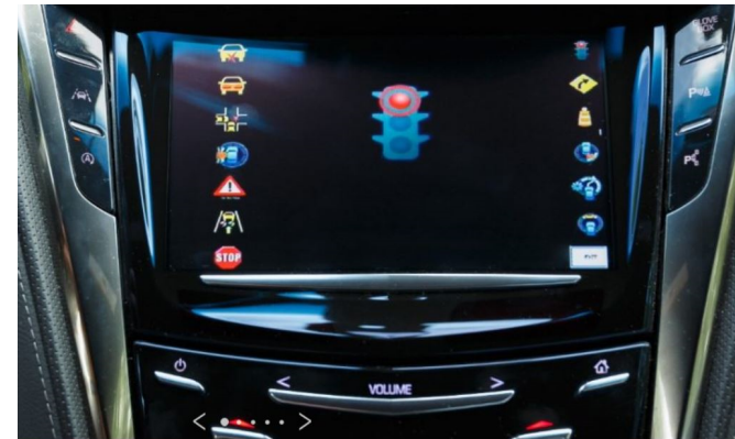
Cadillac CTS with DSCR: V2V & V2I to Traffic Signals
