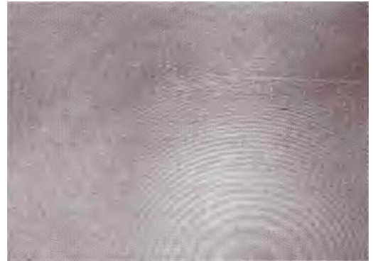
Figure 15: The interference pattern looks like a fingerprint and appears to be random wavy lines, but when a laser is directed at this pattern an apparently 'solid' three-dimensional image appears
