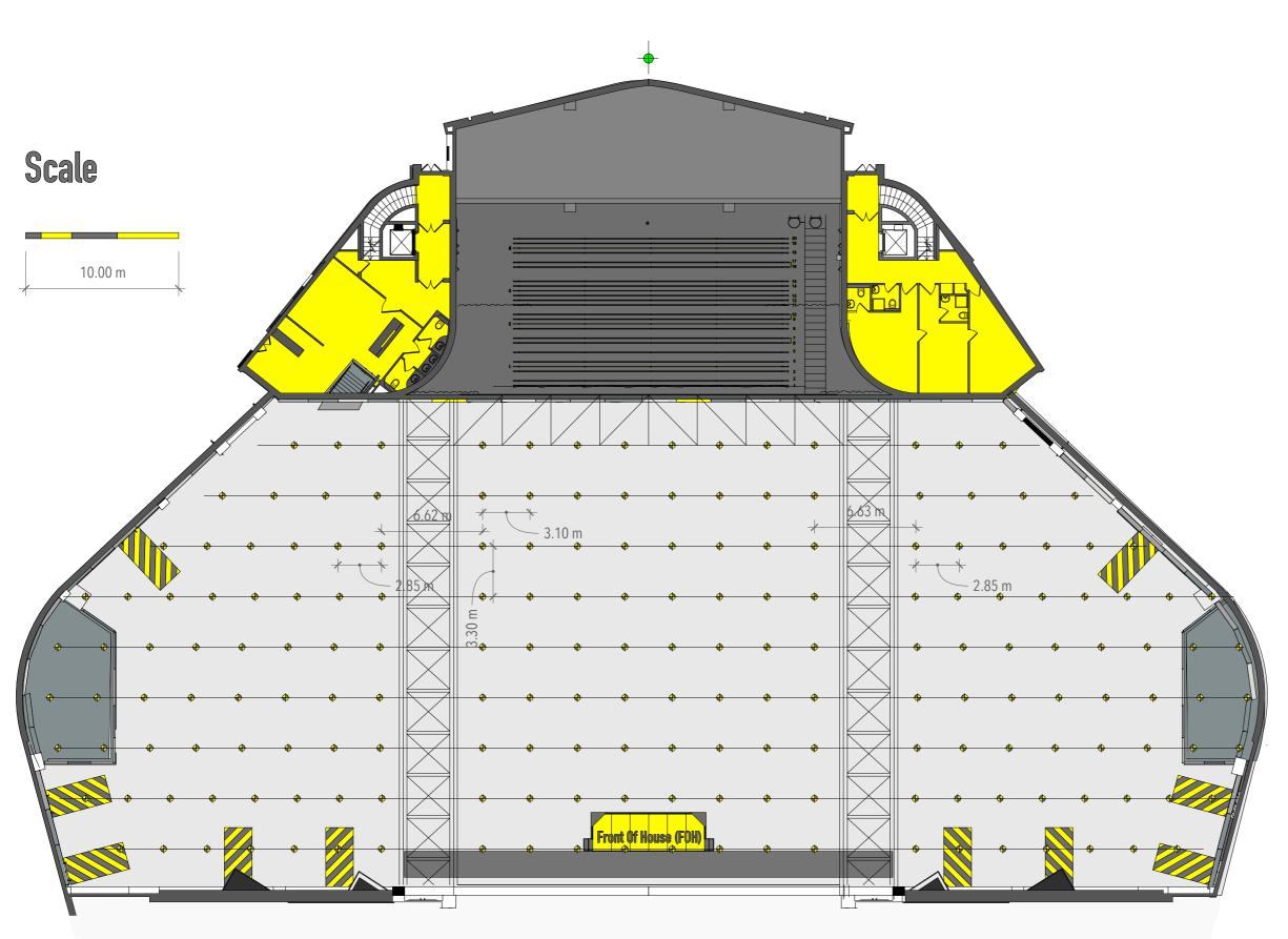
All rigging points to be verified in-field by riggers.
