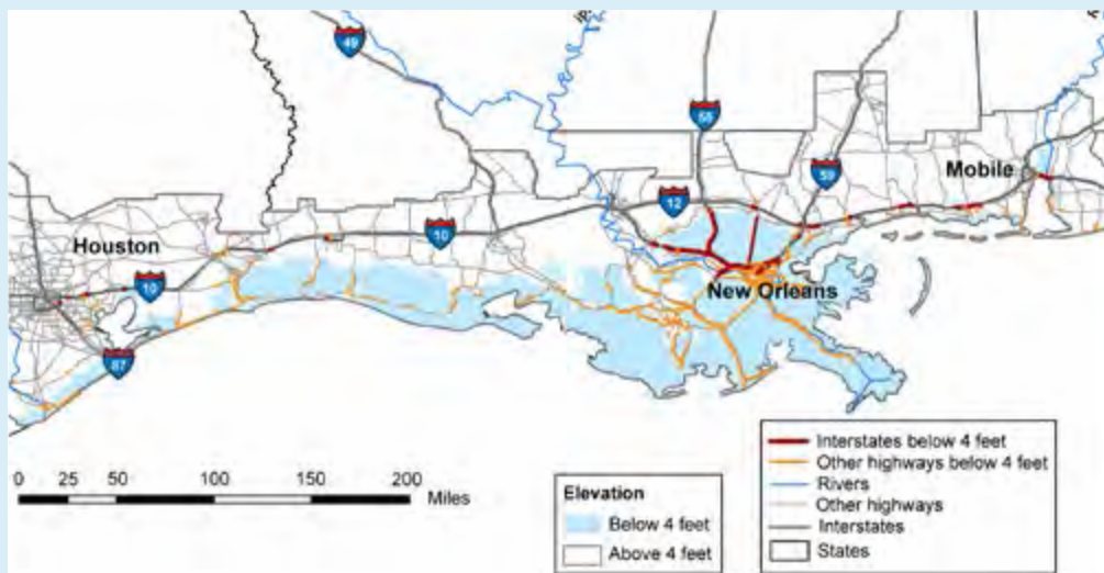
Figure 5.3. Within this century, 2,400 miles of major roadway are projected to be inundated by sea level rise in the Gulf Coast region. The map shows roadways at risk in the event of a sea level rise of about 4 feet, which is within the range of projections for this region in this century (see also Ch. 2: Our Changing Climate, Key Message 10). In total, 24% of interstate highway miles and 28% of secondary road miles in the Gulf Coast region are at elevations below 4 feet. (Figure source: Kafalenos et al. 2008 39 ).
