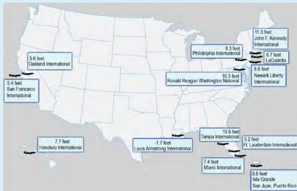
Figure 5.2. Thirteen of the nation's 47 largest airports have at least one runway with an elevation within the reach of moderate to high storm surge. Sea level rise will pose a threat to low-lying infrastructure, such as the airports shown here. (Data from Federal Aviation Administration 2012 33 ).
