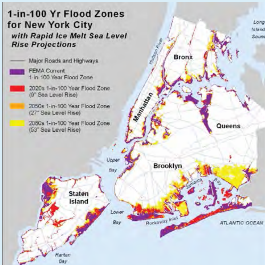
Figure 11.3. Map shows areas in New York's five boroughs that are projected to face increased flooding over the next 70 years, assuming an increased rate of sea level rise from the past century's average. As sea level rises, storm surges reach farther inland. Map does not represent precise flood boundaries, but illustrates projected increases in areas flooded under various sea level rise scenarios. (Figure source: New York City Panel on Climate Change 2013 31 ).
