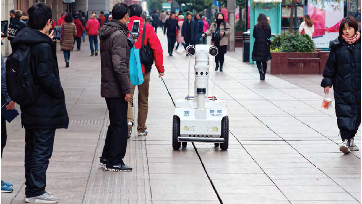
A 5G police robot drives on a sidewalk in China. The robot warns people if they are not wearing masks, checks their body temperature, and scans their face to determine their identity. (atiger/Shutterstock)
