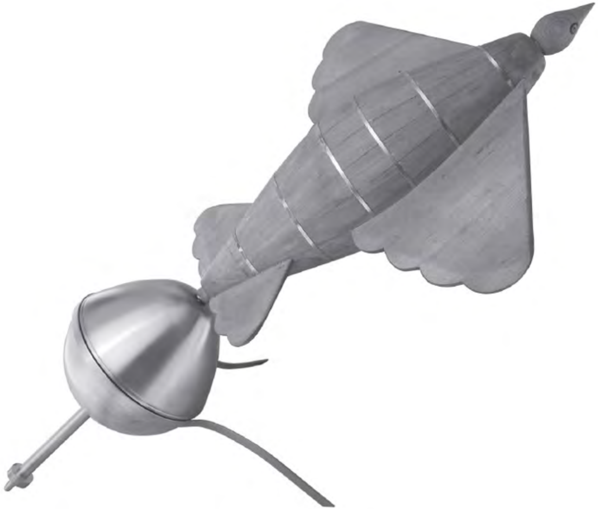
Figure 3.1. A re-creation of Archytas's Pigeon . Compressed air was released, and the Pigeon would be separated from its ignition ball. Image courtesy of the collection and archive of the Kotsanas Museum of Ancient Greek Technology.
