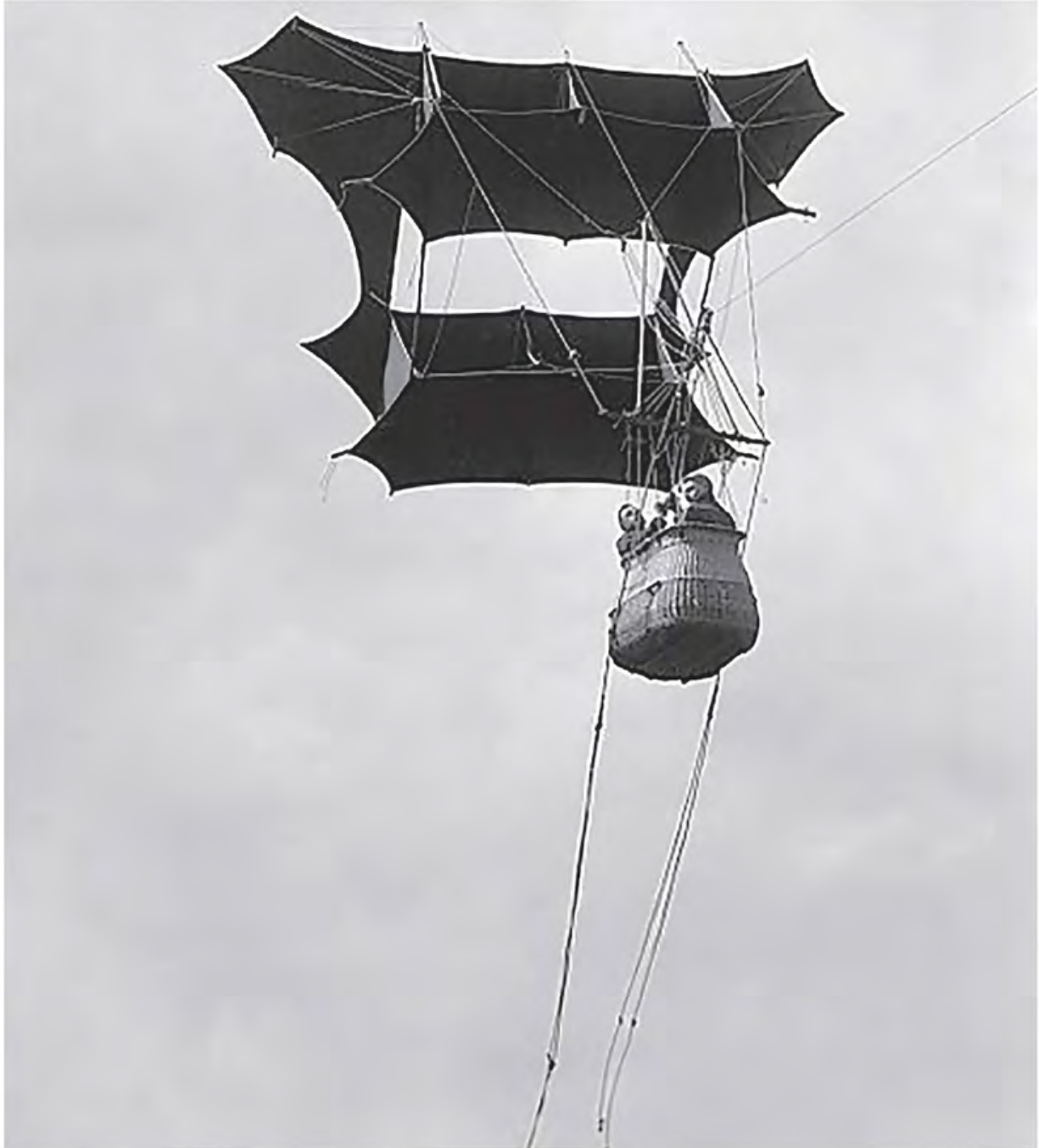
Figure 2.1. During the early twentieth century, the British Army used kites, like this 1908 “Cody war kite” developed by Samuel Franklin “Wild Bill” Cody (better remembered for his traveling Wild West shows), to haul human lookouts into the air for observation purposes. Photo by a Royal Air Force photographer.
